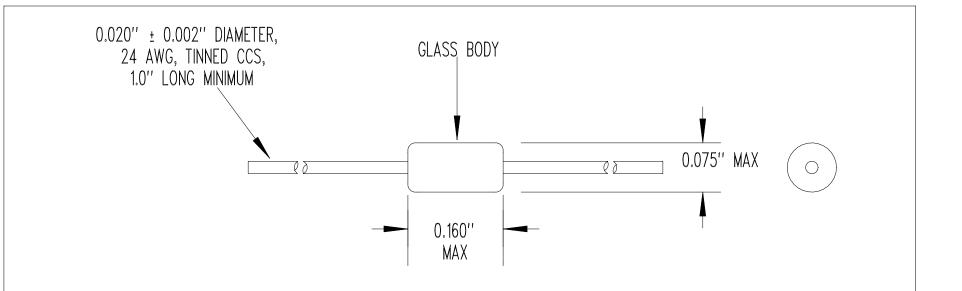
RESISTANCE @  $+25^{\circ}\text{C} = 50,000 \ \Omega \pm 5\%$  RESISTANCE/TEMPERATURE CURVE = "J" BETA "\$" (0 TO  $+50^{\circ}\text{C}) = 3,892^{\circ}\text{K}$  NOMINAL TEMPERATURE COEFFICIENT @  $+25^{\circ}\text{C} = -4.4\%$ °C NOMINAL DISSIPATION CONSTANT = 2 mW/°C NOMINAL (STILL AIR) THERMAL TIME CONSTANT = 5 SECONDS NOMINAL (STILL AIR) THERMAL TIME CONSTANT = 0.5 SECONDS NOMINAL (STIRRED OIL) MAXIMUM TEMPERATURE RATING =  $+300^{\circ}\text{C}$
