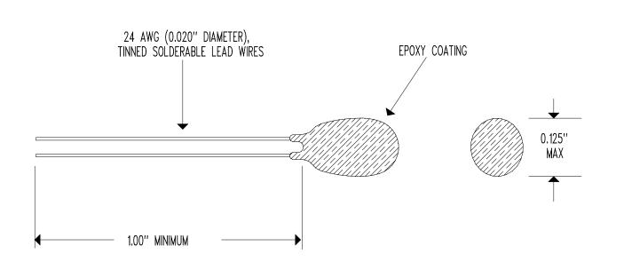
RESISTANCE @  $+25^{\circ}$ C =  $10,000 \Omega \pm 10^{\circ}$ RESISTANCE/TEMPERATURE CURVE = "G" TEMPERATURE COEFFICIENT @  $+25^{\circ}$ C = -4.04%/C NOMINAL BETA " $\beta$ " (0 TO  $+50^{\circ}$ C) =  $3,575^{\circ}$ K NOMINAL DISSIPATION CONSTANT = 3 mW/C NOMINAL THERMAL TIME CONSTANT = 15 SECONDS MAXIMUM (STILL AIR) THERMAL TIME CONSTANT = 2 SECONDS MAXIMUM (WELL STIRRED OIL) MAXIMUM TEMPERATURE RATING =  $+150^{\circ}$ C
