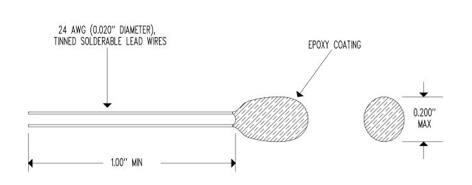
RESISTANCE @  $+25^{\circ}$ C = 300  $\Omega$  ± 10% RESISTANCE/TEMPERATURE CURVE = "F" BETA " $\beta$ " (0 TO  $+50^{\circ}$ C) = 3,419 $^{\circ}$ K NOMINAL TEMPERATURE COEFFICIENT @  $+25^{\circ}$ C = -3.86%/ $^{\circ}$ C NOMINAL DISSIPATION CONSTANT = 3 mW/ $^{\circ}$ C NOMINAL THERMAL TIME CONSTANT = 20 SECONDS NOMINAL MAXIMUM TEMPERATURE RATING =  $+150^{\circ}$ C
