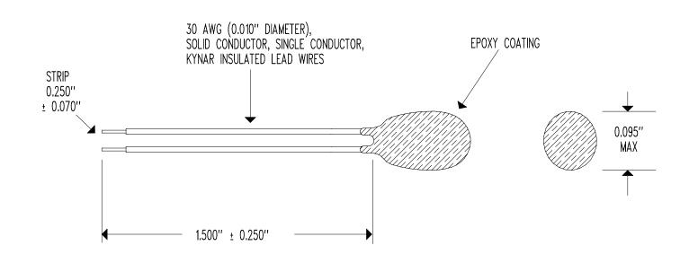
RESISTANCE @  $+25^{\circ}C = 5,000 \Omega$  NOMINAL ACCURACY (0 TO  $+70^{\circ}$ C) = ± 0.10°C RESISTANCE/TEMPERATURE CURVE = "J" TEMPERATURE COEFFICIENT @  $+25^{\circ}C = -4.4\%$ /C NOMINAL BETA " $\beta$ " (0 TO +50°C) = 3,892°K NOMINAL DISSIPATION CONSTANT = 1 mW/°C NOMINAL THERMAL TIME CONSTANT = 10 SECONDS MAXIMUM (STILL AIR)
