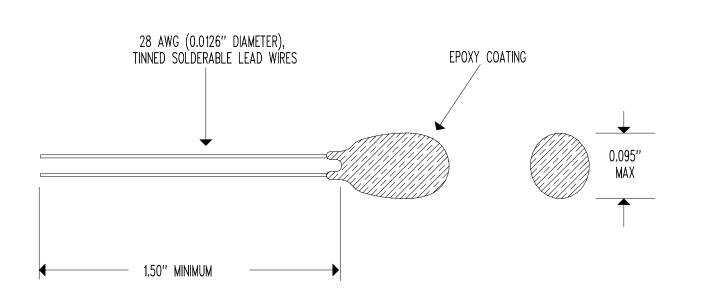
RESISTANCE @  $\pm 25^{\circ}\text{C} = 100,000 \ \Omega \pm 10\%$ RESISTANCE/TEMPERATURE CURVE = "R"
