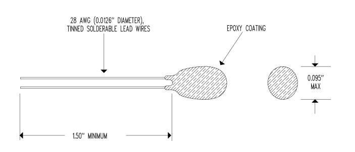
RESISTANCE @  $\pm 25^{\circ}\text{C} = 50,000 \ \Omega \pm 10^{\circ}$  RESISTANCE/TEMPERATURE CURVE = "J" TEMPERATURE COEFFICIENT @  $\pm 25^{\circ}\text{C} = -4.4\%$ /'C NOMINAL BETA " $\beta$ " (0 TO  $\pm 50^{\circ}\text{C}$ ) = 3,892'K NOMINAL DISSIPATION CONSTANT = 1 mW/'C NOMINAL THERMAL TIME CONSTANT = 10 SECONDS MAXIMUM (STILL AIR) THERMAL TIME CONSTANT = 1 SECOND MAXIMUM (WELL STIRRED OIL) MAXIMUM TEMPERATURE RATING =  $\pm 150^{\circ}\text{C}$
