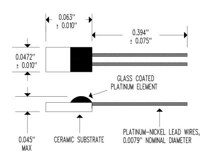
RESISTANCE @ 0°C = 100  $\Omega$  ± 0.06% ACCURACY @ 0°C = ± 0.15°C DIN 43760 ACCURACY CLASS = "A" TCR = 3,850 ppm/°C TEMPERATURE RATING = -200 TO +600°C THERMAL TIME CONSTANT = 1.2 SECONDS NOMINAL (AIR 1 m/SECOND) DISSIPATION CONSTANT = 1.8 mW/°C NOMINAL (AIR)
