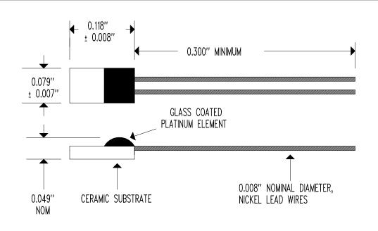
RTD ELEMENT RESISTANCE @ 0°C = 500  $\Omega$  ± 0.12% RTD ELEMENT ACCURACY @ 0°C = ± 0.30°C
