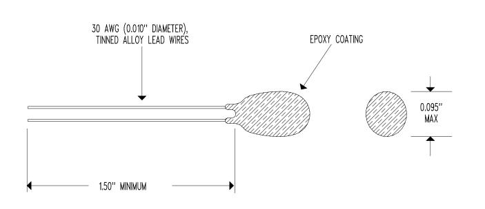
RESISTANCE @  $+25^{\circ}C = 5,000 \ \Omega$  NOMINAL ACCURACY (0 TO  $+70^{\circ}C$ ) =  $\pm$  0.10°C RESISTANCE/TEMPERATURE CURVE = "J" TEMPERATURE COEFFICIENT @  $+25^{\circ}C = -4.4\%$ /°C NOMINAL BETA " $\beta$ " (0 TO  $+50^{\circ}C$ ) = 3,892°K NOMINAL DISSIPATION CONSTANT = 1 mW/°C NOMINAL THERMAL TIME CONSTANT = 10 SECONDS MAXIMUM (STILL AIR) THERMAL TIME CONSTANT = 1 SECOND MAXIMUM (WELL STIRRED OIL) MAXIMUM TEMPERATURE RATING =  $+150^{\circ}C$
