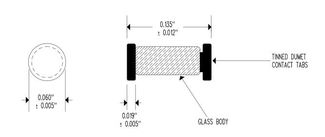
RESISTANCE @  $+25^{\circ}$ C = 1,000  $\Omega$  ± 10% RESISTANCE/TEMPERATURE CURVE = "B" BETA " $\beta$ " (0 TO  $+50^{\circ}$ C) = 2,941 K NOMINAL TEMPERATURE COEFFICIENT @  $+25^{\circ}$ C = -3.31%/C NOMINAL DISSIPATION CONSTANT = 2 mW/C NOMINAL THERMAL TIME CONSTANT = 8 SECONDS NOMINAL MAXIMUM TEMPERATURE RATING =  $+220^{\circ}$ C
