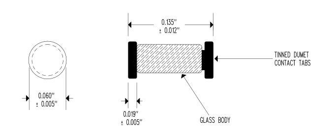
RESISTANCE @  $+25^{\circ}$ C = 50,000  $\Omega$  ± 10% RESISTANCE/TEMPERATURE CURVE = "J" BETA " $\beta$ " (0 TO  $+50^{\circ}$ C) = 3,892°K NOMINAL TEMPERATURE COEFFICIENT @ +25C = -4.4%/°C NOMINAL DISSIPATION CONSTANT = 2 mW/°C NOMINAL THERMAL TIME CONSTANT = 8 SECONDS NOMINAL MAXIMUM TEMPERATURE RATING =  $+220^{\circ}$ C
