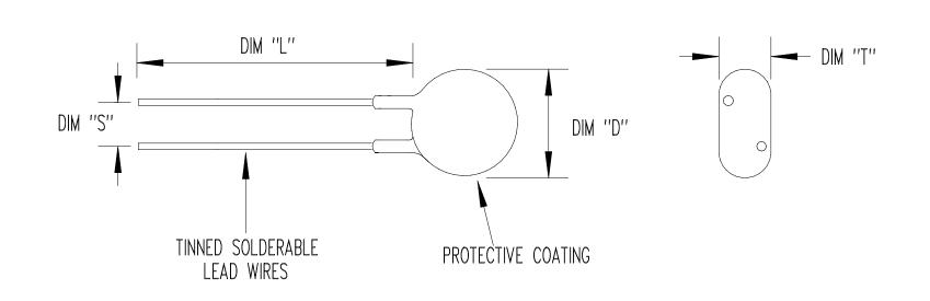
RESISTANCE @  $+25^{\circ}C = 10 \Omega \pm 20^{\circ}$
