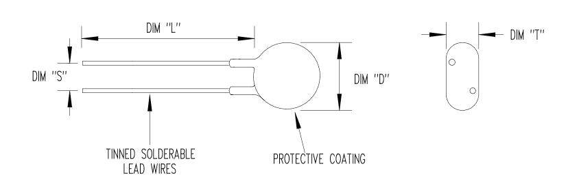
RESISTANCE @  $+25^{\circ}C = 40 \Omega \pm 20^{\circ}$
