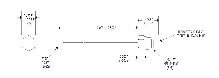
RESISTANCE @  $+25^{\circ}C = 10,000 \Omega \pm 5\%$ RESISTANCE/TEMPERATURE CURVE = "J" TEMPERATURE COEFFICIENT @  $+25^{\circ}C = -4.4\%$ /'C NOMINAL MAXIMUM TEMPERATURE RATING =  $+105^{\circ}C$
