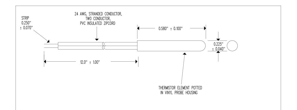
RESISTANCE @  $+25^{\circ}C = 2,252 \Omega$  NOMINAL ACCURACY (0 TO  $+70^{\circ}C$ ) =  $\pm$  0.10°C RESISTANCE/TEMPERATURE CURVE = "J" BETA " $\beta$ " (0 TO  $+50^{\circ}C$ ) = 3,892°K NOMINAL TEMPERATURE COEFFICIENT @  $+25^{\circ}C = -4.4\%$ /°C NOMINAL MAXIMUM TEMPERATURE RATING =  $+105^{\circ}C$
