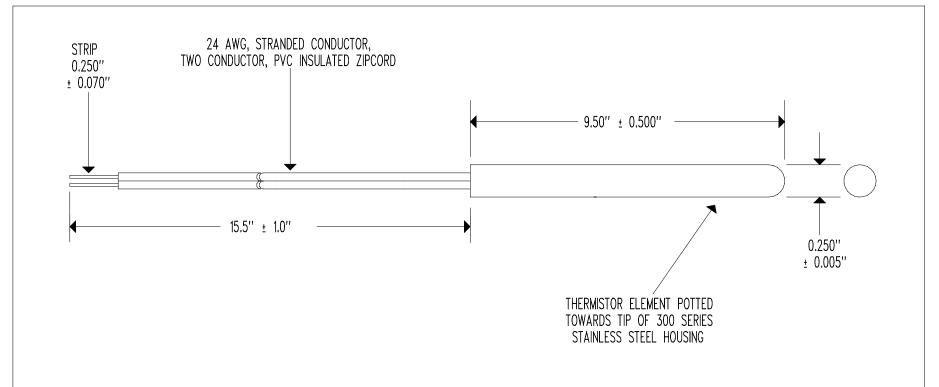
RESISTANCE @  $+25^{\circ}$ C = 10,000  $\Omega$  ± 2% ACCURACY (-20 TO +70°C) = ± 0.01°C OF R-T CHART SUPPLIED WITH PROBE RESISTANCE/TEMPERATURE CURVE = "J" BETA " $\beta$ " (0 TO +50°C) = 3,892°K NOMINAL TEMPERATURE COEFFICIENT @ +25°C = -4.4%/°C NOMINAL MAXIMUM TEMPERATURE RATING = +105°C
