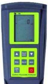
The 706 tests forklift exhaust gases for the presence and location of carbon monoxide leaks. This instrument fits comfortably in your hand and operates with just the push of a
