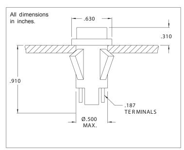
Mounting: Will snap-fit into Ø.500/.505 hole in panels .020/.100 thick. Push-on speednut SN0461 also available. Mounting hole pattern on page SP2.
