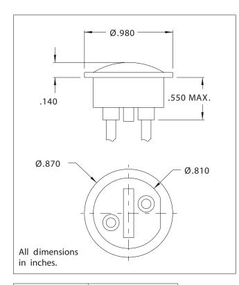
Mounting: Supplied with speednut SN2089. Mounting hole pattern on page SP2.
