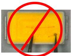
(2) In general, LEDs should only be handled from the side. By the way, this also applies to LEDs without a silicone sealant, since the surface can also become scratched.
