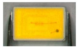
(3) When populating boards in SMT production, there are basically no restrictions regarding the form of the pick and place nozzle, except that mechanical pressure on the surface of the resin must be prevented.
