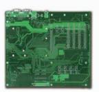
Portwell PCOM-C210 is designed with ATX form factor with COM Express Type II row connectors, suitable for evaluation testing of Portwell's Type 2 COM Express modules on PCI-E, PCI, PEG/SDVO, IDE, SATA, LAN, LVDS, AUDIO, etc. interfaces. We also provide carrier board design guides for your own carrier board development reference.
