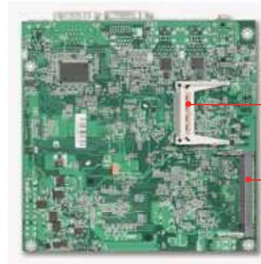
Built with the Intel® mobile 945GSE chipset, WADE-8070 takes advantage of Intel® Atom™ N270 technologies. This low power, fanless WADE-8070 makes it most suitable for POS, Medical, Gaming and Digital Signage applications.
