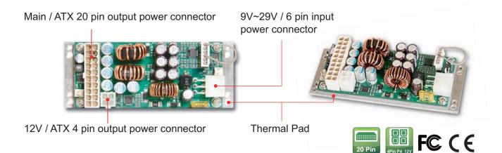
GADIWA- 3161 is a wide input board type converter. It normally support 128Watts and peak 160Watts. GADIWA-3161 can save more space and cost, it's not only capability for fan-less system but also suitability for different application. Besides, the converter is made and tested by automatic production line; therefore, it can provide high quality and performance.
