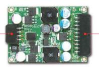
Main / Mini-Fit 20 pin output power connector
