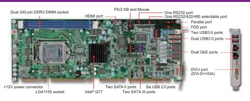
ROBO-8111VG2AR-Q77 is based on Intel® Q77 chipset and Core™ i7/i5 sku processor. It's suitable for Medical, Factory Automation, and Digital Signage applications.
