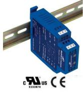
The 232CLDR is a DIN Rail mountable RS-232 to Current Loop Converter. It has one optically isolated 20 mA transmit loop and one optically isolated receive loop. Each loop can be set to either "Active" or "Passive." When set to "Active" an isolated 20 mA current is supplied for each loop (transmit and receive). One 10 to 30 VDC power supply provides power to the converter and both current loops.
