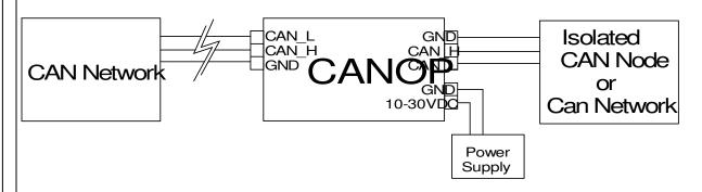
The CAN network must be terminated at both ends according to the CAN specification. Networks not properly terminated may have data errors, or miss the data completely. The CANOP creates two new ends to the CAN network. Space is provided on the board for a termination resistor on each side, R6 and R8. A 120-ohm resistor is recommended for the termination. If the CANOP is not at the end of the network, it should not be terminated.
