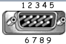
RS-232 Pin-out DB9 Male DTE
