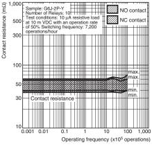
lote: 1. The tests were conducted at an ambient temperature of 23°C.
