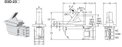
Note: The dimensions OP1 and OP2 apply to the D3D-21□ only. The D3D-22□ and D3D-23□ are SPST-NC and SPST-NO respectively and so therefore have only one corresponding dimension here (OP).
