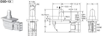
Note: The dimensions OP1 and OP2 apply to the D3D-11□ only. The D3D-12□ and D3D-13□ are SPST-NC and SPST-NO respectively and so therefore have only one corresponding dimension here (OP).
