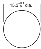
Panel Cutout Dimension Panel thickness = 1 to 4 mm
