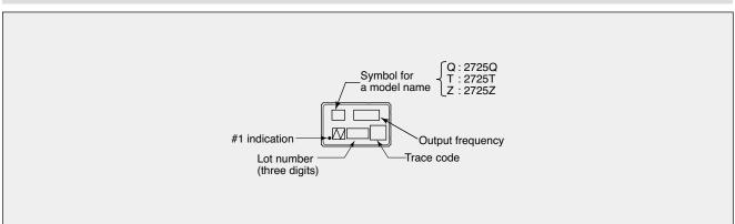
• Because of space limitations, the output frequency is indicated as six digits including the decimal point. Therefore, 14.31818 MHz is indicated as 14.318.
