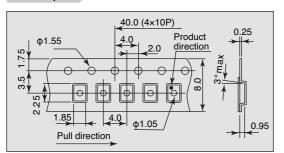
Up to 3,000 pieces per reel are boxed and shipped with the taping method shown above.
