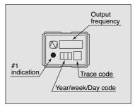
• Because of space limitations, the output frequency is indicated as five digits including the decimal point. Therefore, 28.63636 MHz is indicated as
