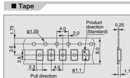
Up to 3,000 pieces per reel are boxed and shipped with the taping method shown above.
