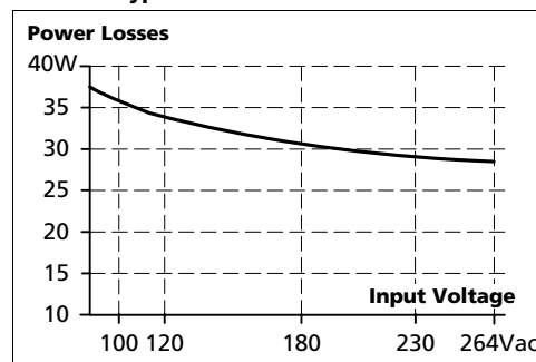
Fig. 9-4 Losses vs. input voltage at 12V, 30A, typ.
