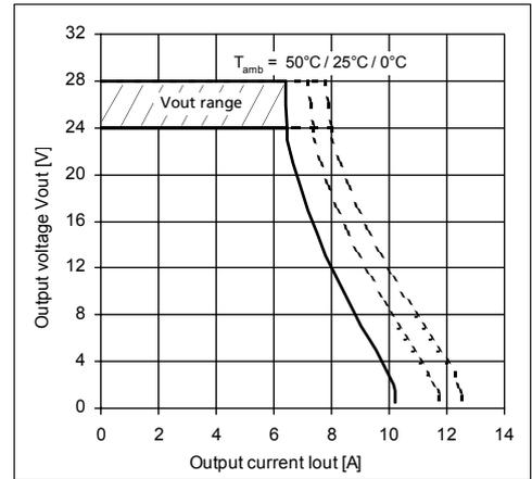
**Output current over input voltage (min., at V<sub>out</sub>=24V)**
