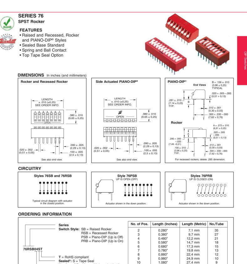
\*A top tape seal is required for switches that are machine soldered or heavily cleaned after hand soldering. To order top seal versions, add "S" to the Grayhill part number.
