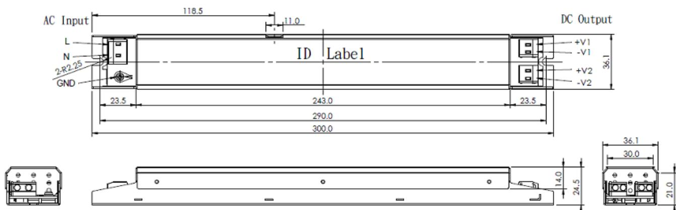
Input Connector: WAGO 235-502 2Pin or Equivalent
