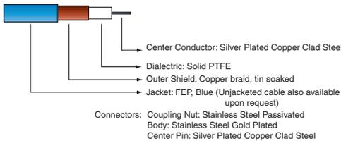
Center Conductor: Silver Plated Copper Clad Steel
