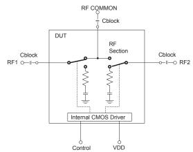
Cblock should be free of resonance over frequency of operation.
