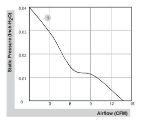
Air Flow-Static Pressure Characteristics
