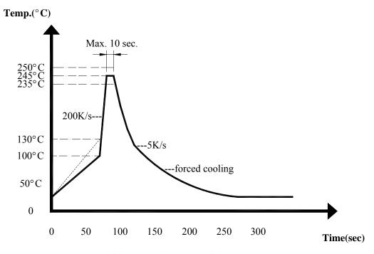
Recommendable wave soldering condition is as follows.
