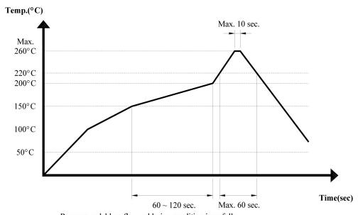
Recommendable reflow soldering condition is as follows.
