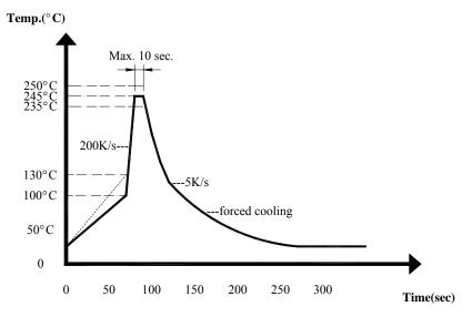
Recommendable wave soldering condition is as follows. Note 1: It is requested that wave soldering should be executed after heat of product goes down to normal temperature. Note 2: Peak wave temperature of  $235^{\circ}\text{C} \sim 250^{\circ}\text{C}$  maximum of 10 sec. .
