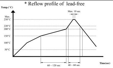
Recommendable reflow soldering condition is as follows.
