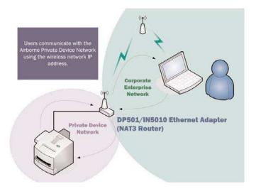
The Ethernet Adapter from Quatech includes a fully functional Network Address Translation (NAT) router. When coupled with the built-in DHCP server on the Ethernet port the most powerful Ethernet adapter in the M2M market comes to life. Your Ethernet device needs no special security settings, IP configuration or proprietary protocols. If it supports DHCP or Static IP addressing you can quickly connect to the most advanced Enterprise class networks without changing your platform.
