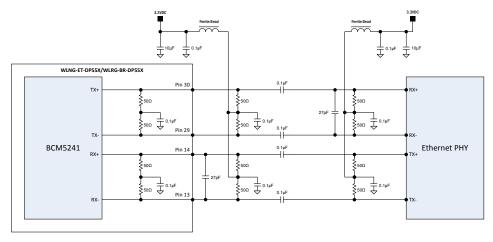
Historically, using auto-negotiate, with a capacitive coupling network has been difficult. Quatech recommends that auto-negotiate not be used when implemented with the DP550 devices. The Ethernet mode can be set via the web interface via the **Configuration**| **Ethernet Settings**| **Ethernet Port Speed/Duplex** field or through the CLI interface using the **eth-mode** command.
