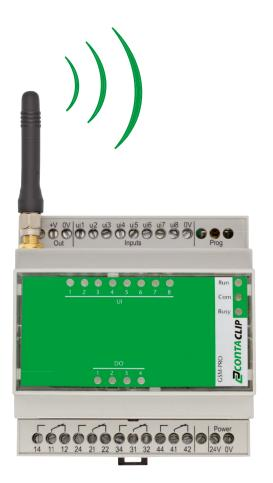
The GSM-PRO module features eight multi-function inputs. The input module may be selected as either digital (24 V DC) or analogue (0 to 10V), so that many different signal levels can be connected.
