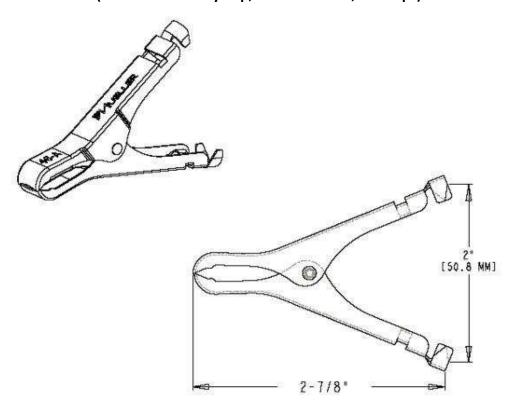
Dimensions: Length: 2.88" (73 mm); Width: .48" (12 mm); Height: 2" (51 mm)
