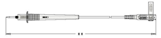
Multiple Feature Test Prod to Right Angle Shrouded Banana
